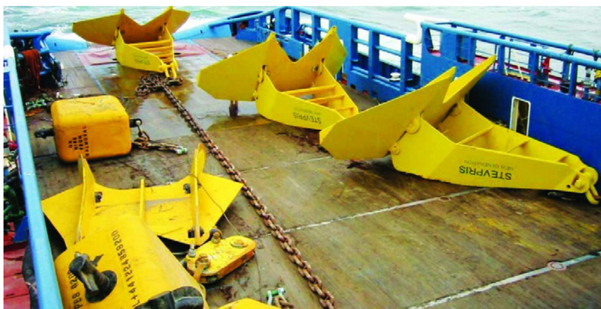
Figure 13: Drag embedment anchors on the deck of an anchor handling vessel (Vryhof, 2020)
