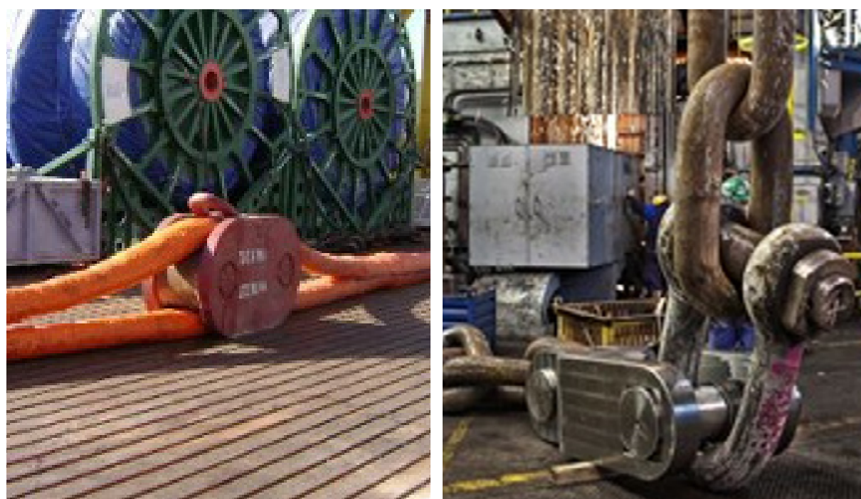
Figure 19: H-shackle (L) (Intermoor, 2021) and D-shackle (R) (EDP, n.d.)
