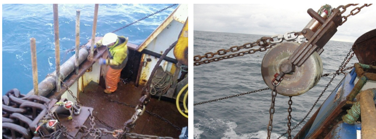
Figure 5: Chain link clump weight and roller ball clump weights (Source: John Watt, 2020)
