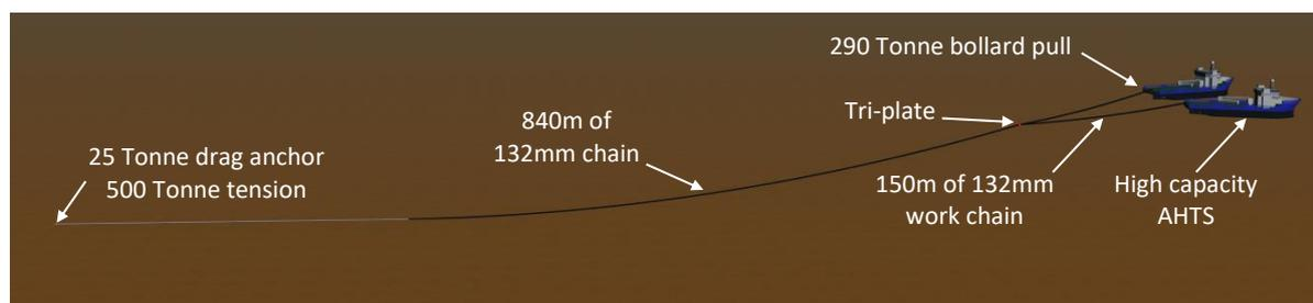
Figure 22 – Drag anchor test tensioning load path
