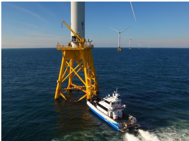
Figure 1: Crew Transfer Vessel Push on Process [3]
