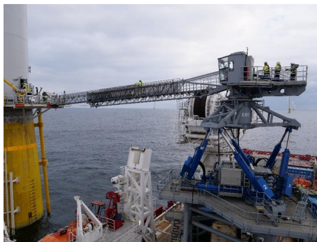
Figure 3: Walk-to-Work Gangway reaching to a floating turbine, courtesy of Ampelmann
