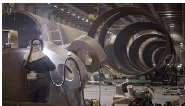
Figure 5 Can sections and cylindrical sections at Welcon® factory [10]
