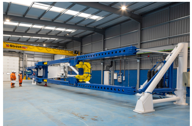
Figure 13 - Dynamic cable test rig (credit: ORE Catapult)
