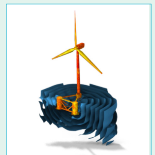
Figure 35 - Modelled structure of Kincardine substructure to model how sound radiates off steel surfaces
