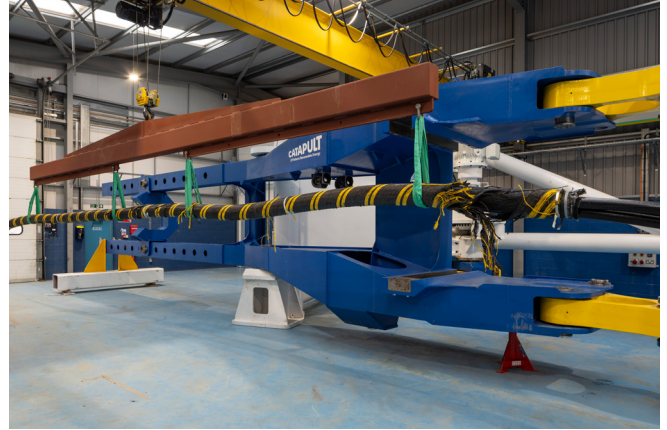
Figure 25 - Dynamic cable test rig at the Floating Wind Innovation Centre in Aberdeen (credit: ORE Catapult)
