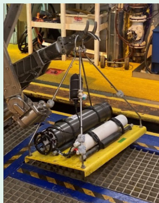
Figure 34 - Recorders being deployed at Kincardine (courtesy of JASCO Applied Sciences)
